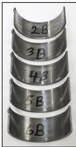
Above left: The rod and main bearings show no sign of "grabbing" from the loss of oil pressure.
